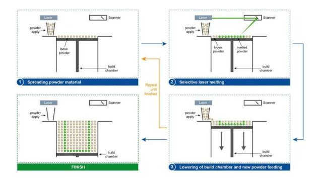
Additive manufacturing process can be summarized using a few points including:
